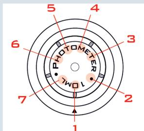
6. After successful indexing, the cuvette lid, the smallest indexed value and the index of the ideal position are shown in green on the display. Mark the cuvette (not the lid!) at the position of the index of the ideal position, e.g. with a waterproof pen. Important: Place your mark above the 10ml line, otherwise the mark will influence your measurement! Press "Done".
