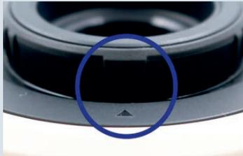
*\*It is possible that there is no arrow on the adapter yet. This will only appear on upcoming models. If your model does not have a triangle, please make sure that the arrow on the device points to the elevation on the side of the adapter.*
